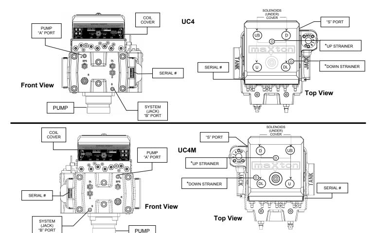
ATTENTION: All Maxton Valves **MUST** be installed with the solenoids in the upright (vertical) position.
