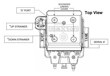
\* Strainer access is provided from the top of the control plate.
