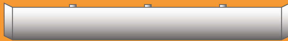
Bumper rails (SS #4 Flat Bar 6" x 1/4")
