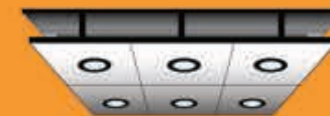
LED downlights in stainless steel drop ceiling
