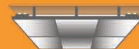
Drop ceiling with perimeter lights
