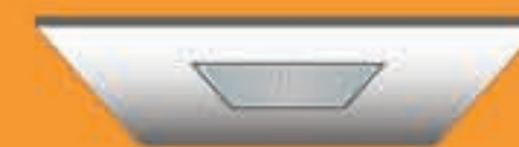
LED lights recessed in canopy
